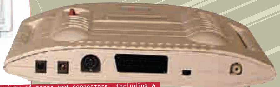
The GX4000 featured a variety of ports and connectors, including a forward-thinking SCART connection
